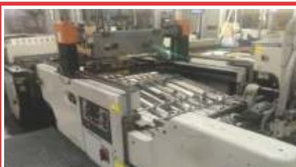
2005 SAKURAI MS 72 A II Automatic High Speed Screen Cylinder Press Maximum Sheet Size: 720 x 520mm, Speed: 3,600 SPH, Printable Thickness (mm) 0.1 - 0.8, Automatic Rear pick-up feeder, Trumax UV Dryer, Ref: 7702
