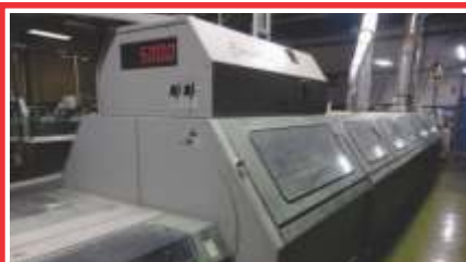
2003 MULLER MARTINI CORONA C15 PERFECT BINDER 15 Feeders, Log Loaders, Corona C15 Binder, Cover Feeder Computer Setting, Signature Recognition, Drying Conveyor, Zenith 3 Knife Trimmer, Ref: 7649
