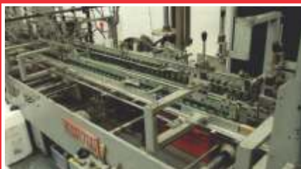
1996 VEGA 700 FOLDING CARTON GLUER To produce sideseam and lockbottom cartons, Lockbottom hooks and former plates, Pafra APC electronic glue system with 2 guns, Batch counter/kicker and totaliser, Compression/delivery section, Ref: 11412
