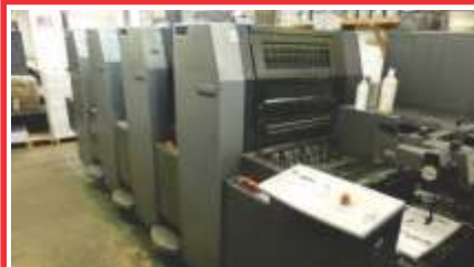
2001 HEIDELBERG SM 52 4 Impressions 129, Maximum Sheet Size 460mm X 520mm, CPC 1-04, CP Tronic, Alcolor, Technotrans Chiller, AutoPlate, Automatic Washups, Powder Spray, Ref: 7695
