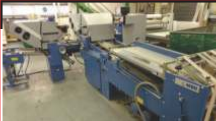
2005 MBO T530 4/4 FOLDER Maximum Sheet Size: 530 x 730 mm, Minimum size 105 x 105 cm, Round Pile Feeder, MBO Ms Controls, Fold Unit 1 4 Plates, Fold Unit 2 4 Plates, Slitting & Scoring, A56 DC Mobile Delivery, Ref: 7149
