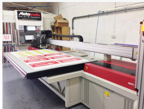
AGFA Jeti 1224 HDC FTR fastest photorealistic industrial grade Flat-To-Roll display graphics printer
